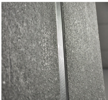
Infused graphite particles give the panel its high insulation value and its 'shine'.
